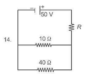
In above circuit if current through 10  $\Omega$  resistor is 2.5 A, value of R is \_\_\_\_\_.
