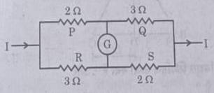
Reason (R): For a balanced bridge small current should flow through the galvanometer.
