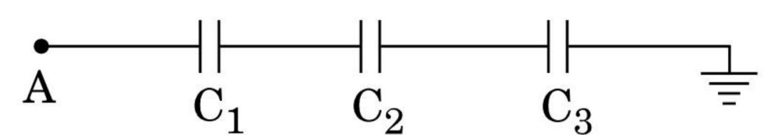
Calculate the potential difference and the energy stored in the capacitor  $C_2$  in the circuit shown in the figure. Given potential at A is 90 V,  $C_1$  = 20  $\mu F$ ,  $C_2$  = 30  $\mu F$  and  $C_3$  = 15  $\mu F$ .
