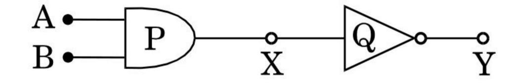
Name the equivalent gate representing this circuit and write its logic symbol.
