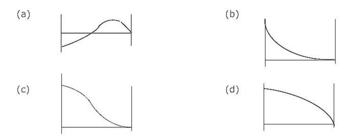
46. A cantilever beam has the square cross section of 10 mm× 10 mm. It carries a transverse load of 10 N. considering only the bottom fibres of the beam, the correct representation of the longitudinal variation of the bending stress is
