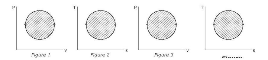
According to the first law of thermodynamics, equal areas are enclosed by
