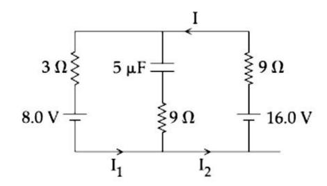
How much is the current I in the circuit in steady state?
