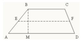
Here AD || BC. Parallel sides are called bases of a trapezoid, the two others (AB and CD) are called lateral sides. A distance between bases (BM) is a height. The segment EF, joining midpoints E and F of the lateral sides, is called a midline of a trapezoid. A midline of a trapezoid is equal to a half-sum of bases:
