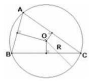
In the figure above, the perpendicular bisectors of the sides AB, BC and CA of triangle ABC meet at O, the circumcentre (centre of the circle passing through the three vertices) of triangle ABC. In Above figure, O is the centre of the circle and BC is a chord. Therefore, the angle subtended at the centre by BC will be twice the angle subtended anywhere else in the same segment.
