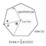
Each side of a regular polygon subtends an angle  $\Theta = 360$  at the centre, as shown in the figure.
