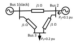
Q.54 The voltage phase angles in rad at buses 2 and 3 are
