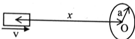
A small bar magnet of dipole moment  $M$  is moving with speed  $v$  along  $x$  direction towards a small closed circular conducting loop of radius ' $a$ ' with its centre  $O$  at  $x = 0$  (see figure). Assume  $x \gg a$  and the coil has a resistance  $R$ . Then which of the following statement(s) is/are true ?
