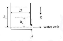
Q. 21 Water discharges steadily from a large reservoir through a long pipeline, as shown in the figure. The Darcy friction factor in the pipe is 0.02. The pipe diameter is 20 cm and the discharge of water is 360 m<sup>3</sup>/h. Water level in the reservoir is 10 m and acceleration due to gravity  $g = 10 \text{ m/s}^2$ . If minor losses are negligible, the length L (in meters, up to one decimal place) of the pipeline is
