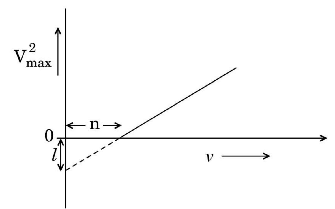
Use Einstein's photoelectric equation to find the expressions for (i) Planck's constant and (ii) work function of the given photosensitive material, in terms of the parameters l, n and mass m of the electron.
