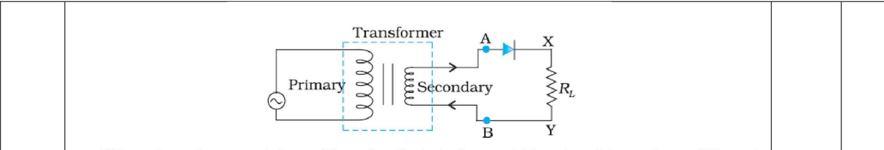
When the voltage at A is positive, the diode is forward biased and it conducts. When A is negative, the diode is reverse-biased and it does not conduct. The reverse saturation current of a diode is negligible and can be considered equal to zero for practical purposes. Thus output is obtain only during positive half cycle. (Note :- Give full credit of explanation if a student just draws input and output waveform.)
