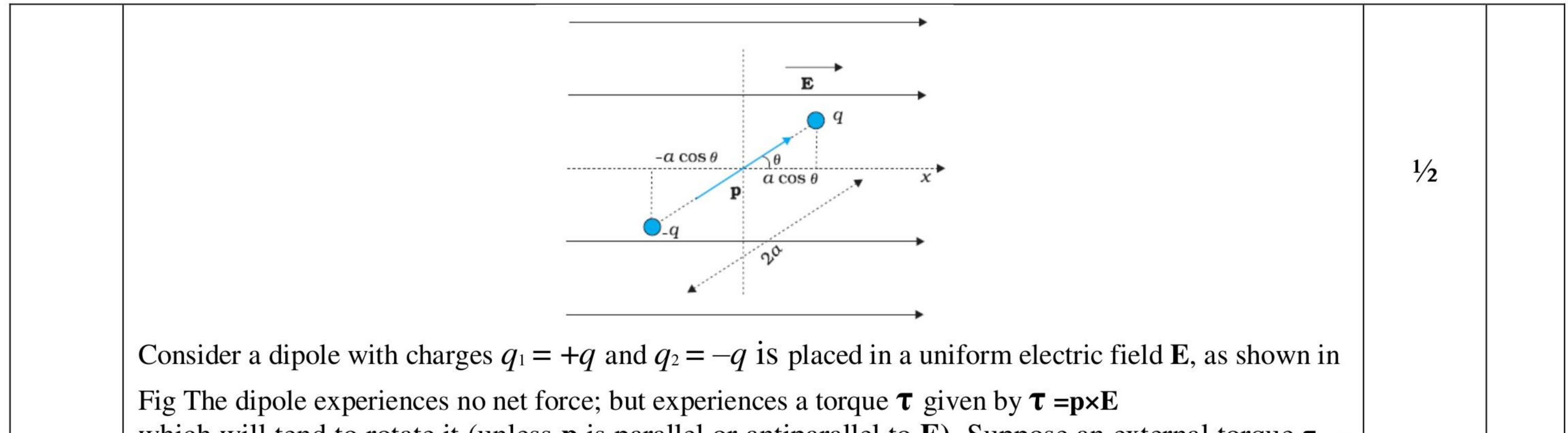
which will tend to rotate it (unless p is parallel or antiparallel to E). Suppose an external torque  $\tau_{ext}$ is applied in such a manner that it just neutralizes this torque and rotates it in the plane of paper from
