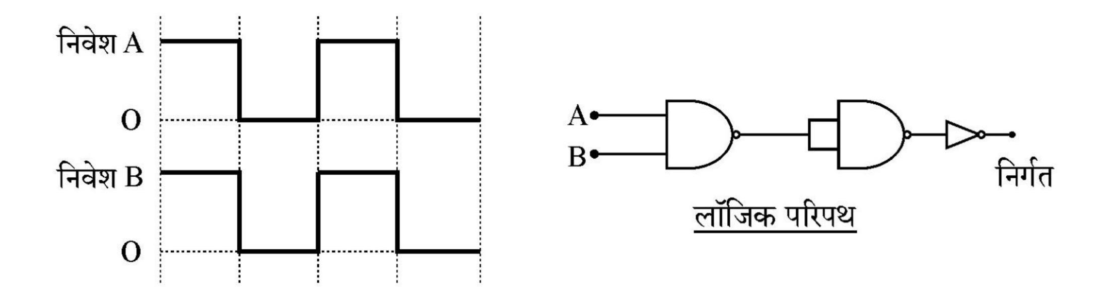
Using the wave forms of the input A and B, draw the output waveform of the given logic circuit. Identify the logic gate obtained. Write also the truth table.
