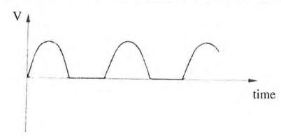
D) If C = 0 and L = 0 and the resistance is connected to an a.c source of frequency f, power varies at twice the frequency (about a constant value) of either V or I.
