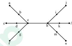
Using the property of eccentricity of a vertex, find every vertex that is the centre of the given tree.
