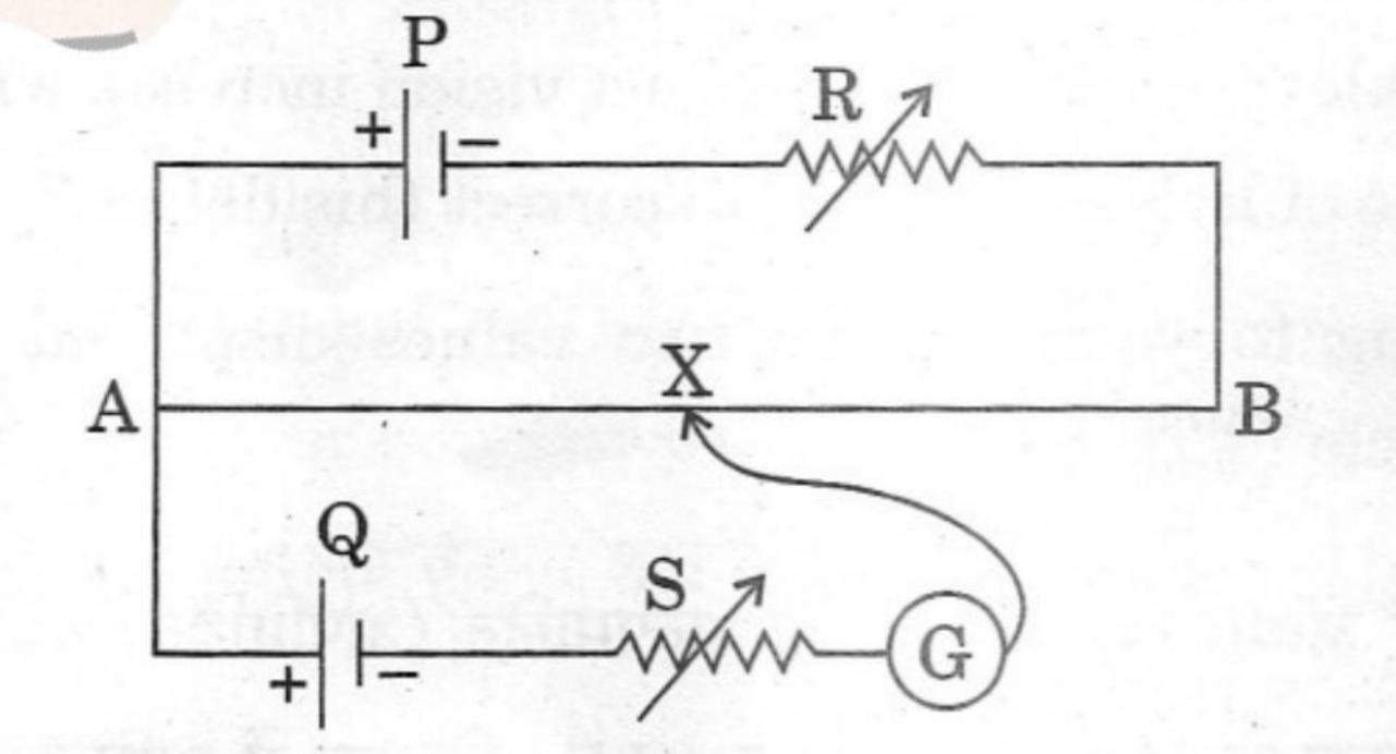
In the potentiometer circuit shown in the figure, the balance point is at X.
