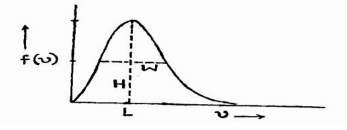
In the figure, H is the height of the peak, L is the location of the maximum and W is the width at half height. As the temperature is decreased,
