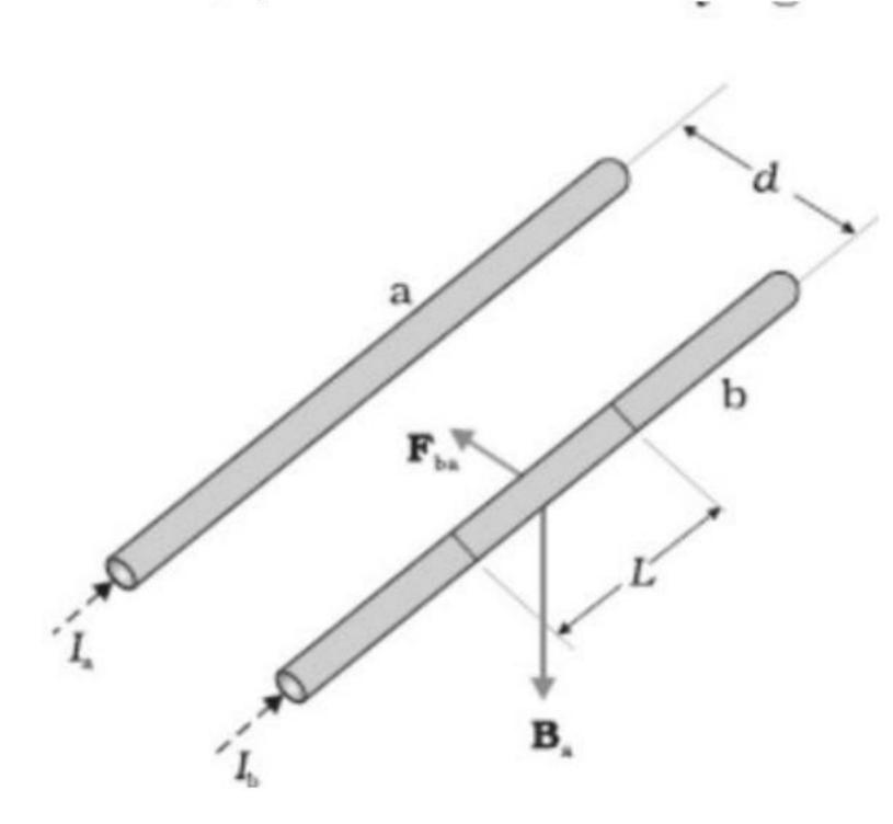
The magnetic field at any point on the wire (b) due to the current in wire (a) is is perpendicular to the plane of two wires and pointing inwards and hence force on it will be towards wire (a). Similarly force on wire (a) will be towards wire (b). Hence two wires carrying currents in same direction attract each other.
