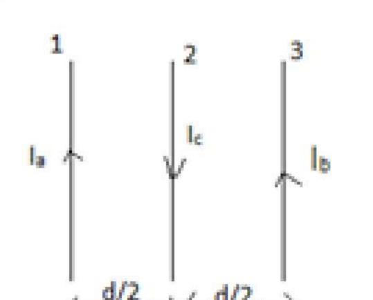
Force on wire (3) due to wire (1)  $= \frac{\mu_0 I_a I_c}{1}$ towards right
