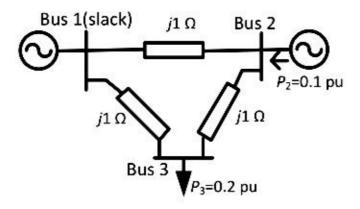
Q.52 The voltage phase angles in rad at buses 2 and 3 are
