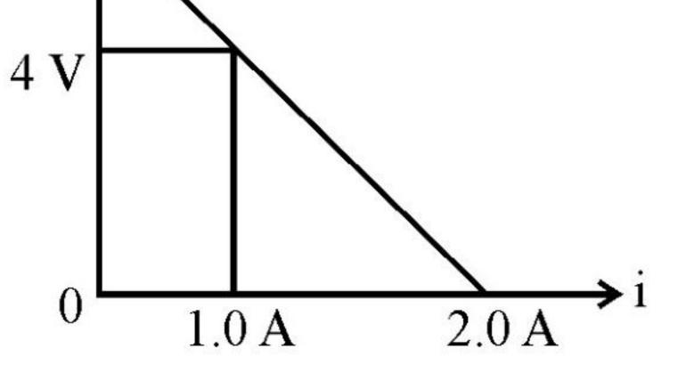
The figure shows a plot of terminal voltage 'V' versus the current 'i' of a given cell. Calculate from the graph (a) emf of the cell and (b) internal resistance of the cell.
