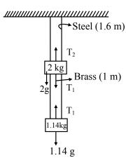
Elongation in steel wire  $\Delta L = \frac{T_2 L}{Av}$
